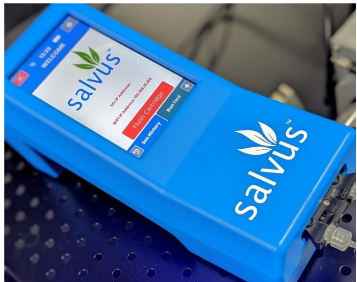
Figure 1: Commercially ready handheld Salvus technology device Sizing and basic layout of the handheld device capable of swapping out cartridges to detect chemical and biological targets in fluid media. Users simply insert the cartridge, introduce sample, and use the touchscreen to run the necessary test parameters to receive qualitative or quantitative analyte results in minutes.
